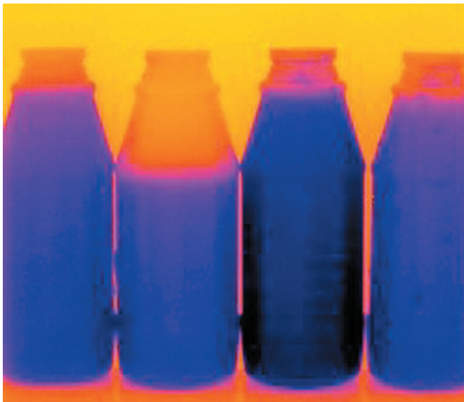
This thermal image shows bottles being filled automatically, so bottles that are over-or under-filled can be removed. If a bottle or jar is made of dark colored glass or plastic thermal imaging cameras are much more effective than visible light cameras.
