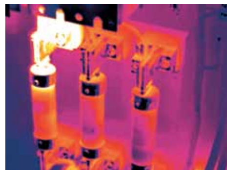
The FLIR T-Series thermal imaging cameras can be used for more than solar module inspections alone; at SOLON these cameras are used to inspect the entire solar installation, including cables, connectors, fuse boxes and inverters, in other words: the entire system.
