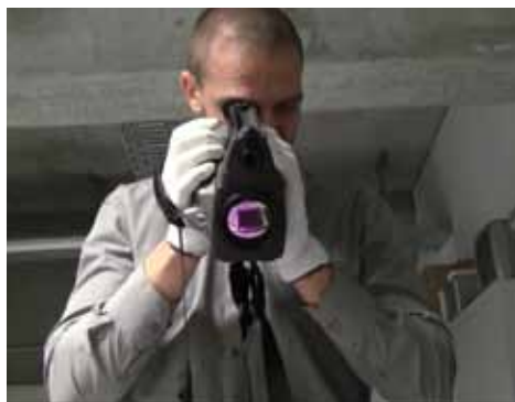
Oliver Frank, Team Manager R&D at SOLON, performs a shunt check using a FLIR thermal imaging camera.
