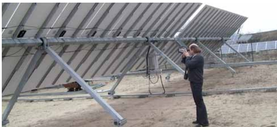
Volker Denzler, thermography expert at SOLON's after sales services department, takes thermal images from the back of a module to avoid reflections.
