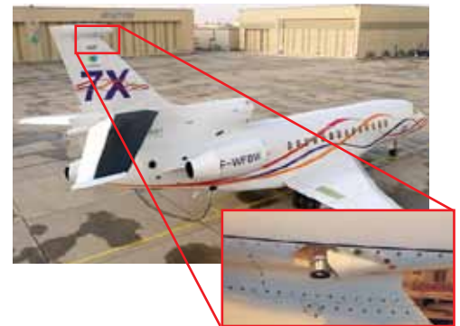
The FLIR SC7750L thermal imaging camera was mounted in the top of the tail of the Falcon 7X, looking down on the right horizontal stabilizer.
