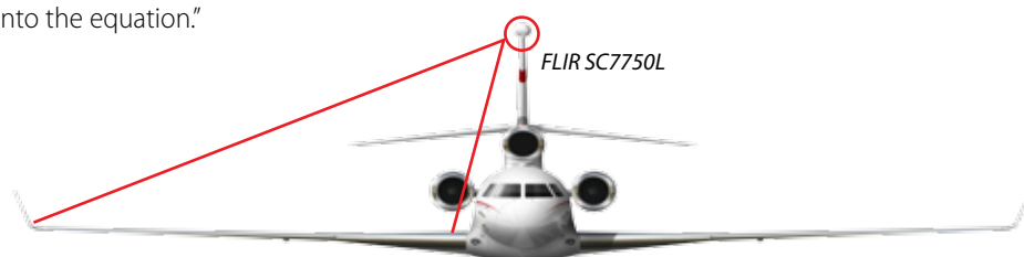
Schematic of the Falcon 7X with the FLIR SC7750L thermal imaging camera mounted in the top of the tail, looking down on the right horizontal stabilizer.
