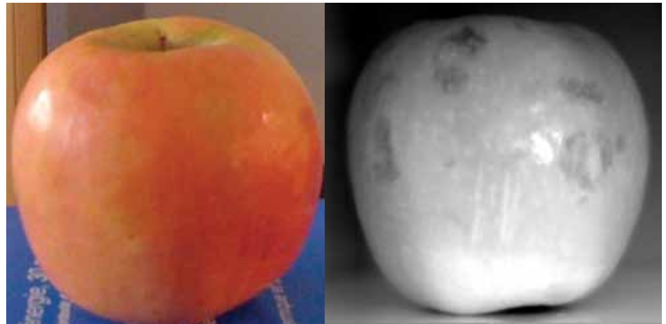
Figure 7. NIR cameras are widely used for inspections and bruise detection in the food industry.
