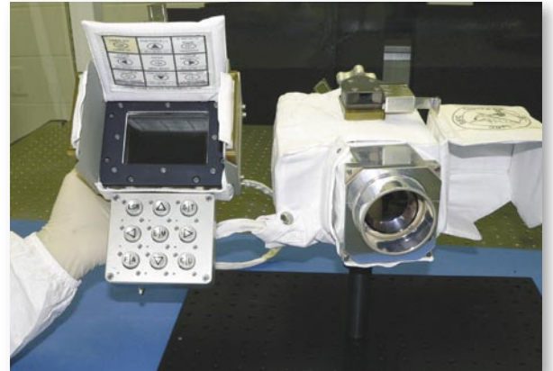
The protective housing for the ThermoCAM S65 as developed by NASA
