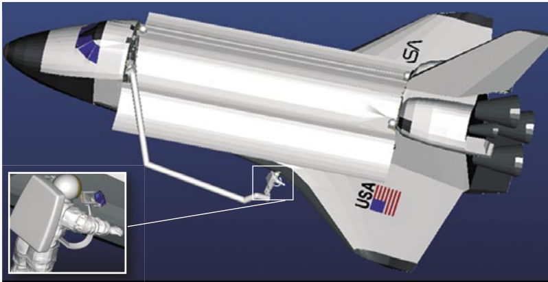
During a spacewalk an astronaut searches with the ThermoCAM S65 for damages at the wing-leading edge.
