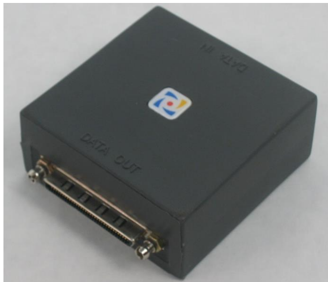
Figure 2-3: Digital Data Serial-to-Parallel Module or SIPO (Part Number: 333-0008-00)
