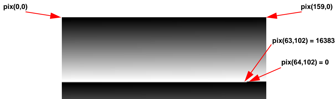
Figure 3-5: Ramp test pattern example for 160 x 128 format sensor (Digital values shown apply to the optional 14-bit digital data stream.)
